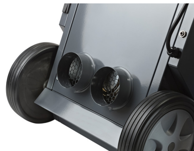
CDT 30 S and CDT 40 S are fitted with a 1 kW heating element, a high pressure fan and two duct spigots, allowing connection of two flexible air ducts Ø100, each up to 5 m long.
